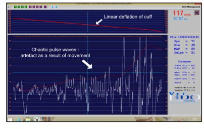
If the above criteria are not met (most commonly the pulse waves will show significant distortion) the reading should be discarded as movement or some other artefact may have affected the accuracy of the blood pressures recorded.
